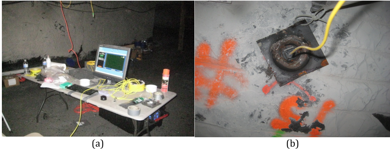
Figure 7: (a) The extensive monitoring equipment needed. (b) The installed instrumented rock bolts with the optical fiber leads.
