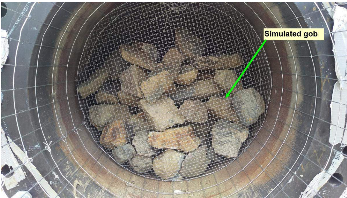
Figure 23. Rock rubble insert for simulated gob experiments in explosion flame reactor (71 cm)
