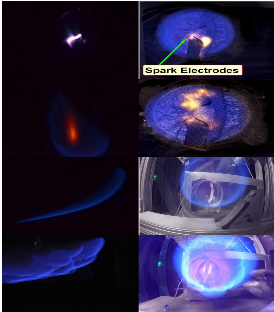
Figure 29. Methane ignition, and transition from spherical flame kernel to turbulent flame (left-images provide side profile view; right-image provide axial view). From top to bottom, we have
