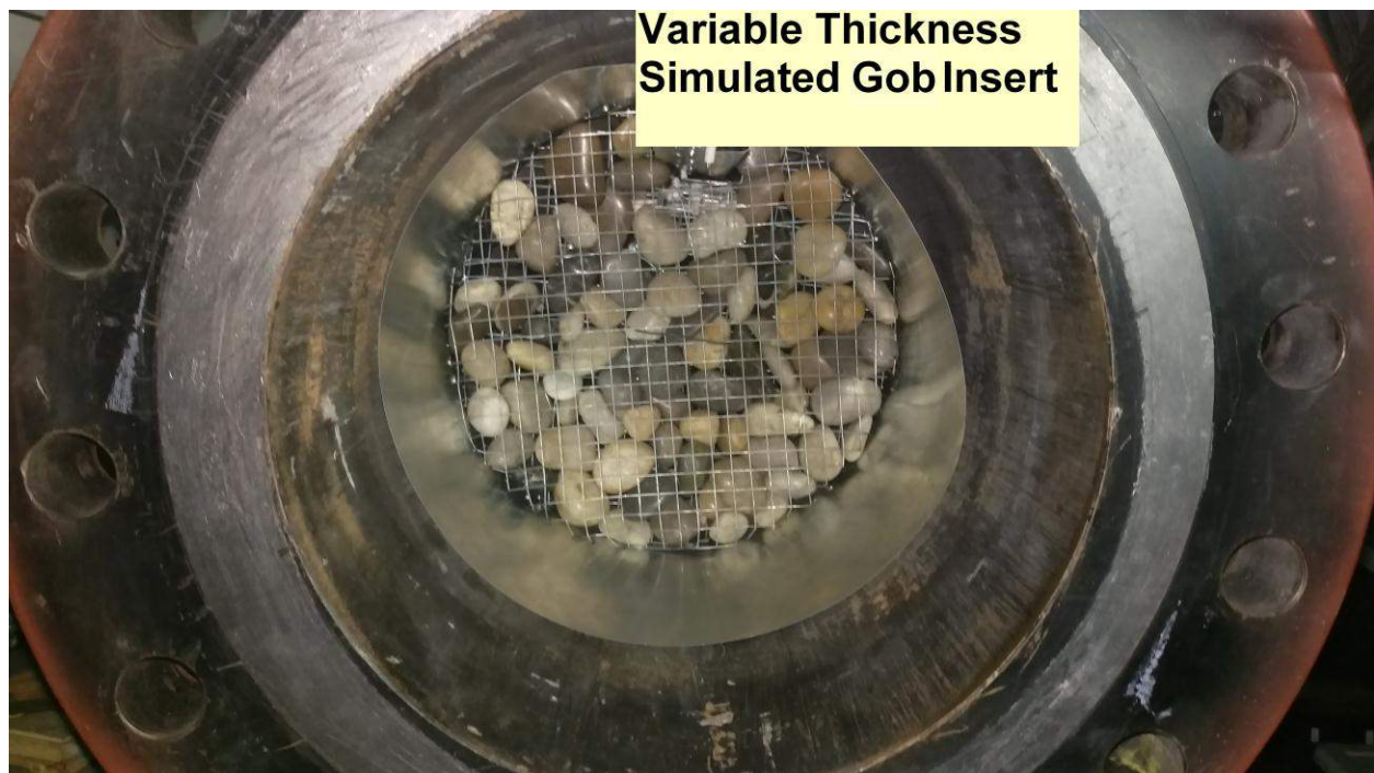
Figure 22. Rock rubble insert for simulated gob experiments in high pressure reactor (30.5 cm )
