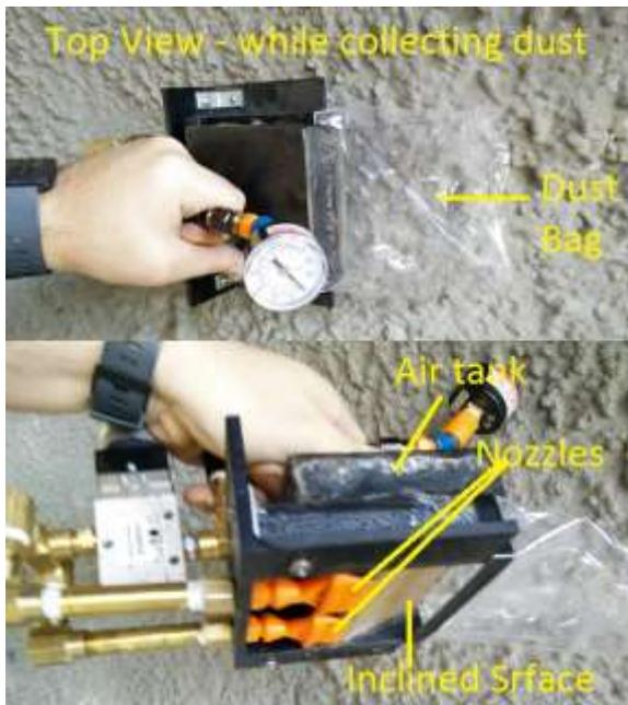
Figure 2: Prototype of the DSD used for experimental testing.
