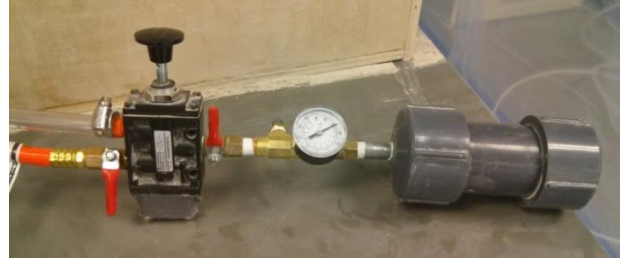
Fig. 2. Palm button charge and release valve system with air vessel.
