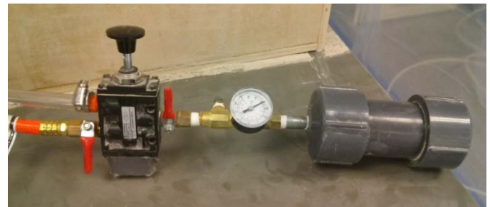
Figure 2. Palm button charge and release valve system.
