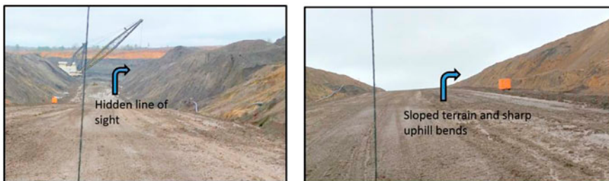
Figure 1. Topology at surface mine with sloped terrain and sharp hairpin bends (the figure on left shows a spoil pile causing hidden line of sight for the 802.11 radio while the figure on the right illustrates sloped terrain and the partial line of sight).
