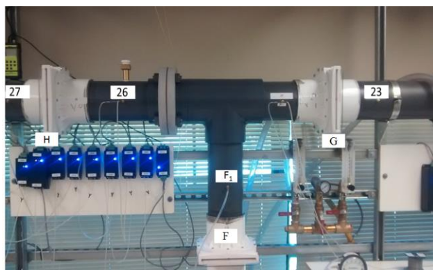
Figure 2: Pressure and velocity transducers installed in the simulated gob area
