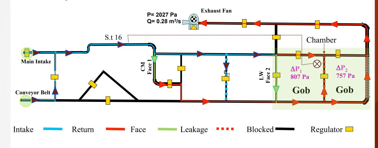
Flow-Through Exhaust System (Mine B)
