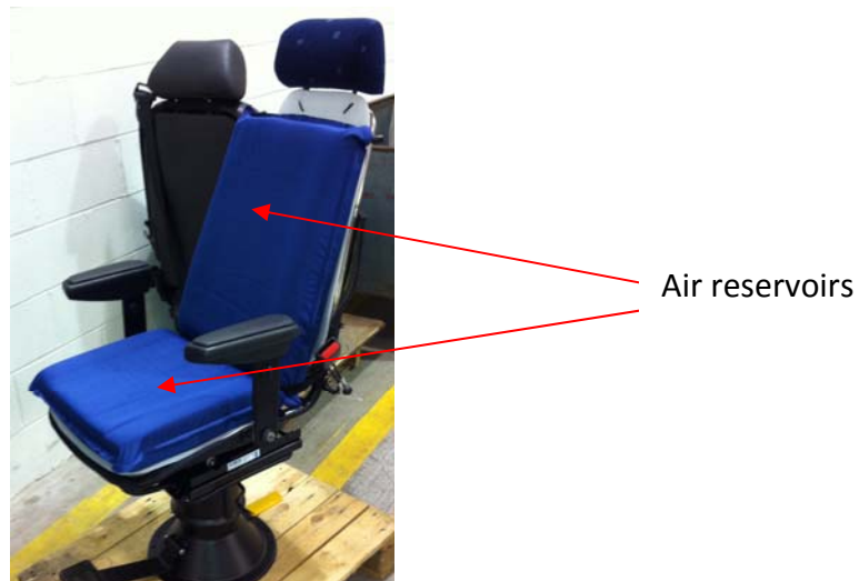
Figure 7. Air-filled bladder with two reservoirs (one on the back and one on the pad) installed on a seat. The air at the seat pan reservoir is blown out to the seat back reservoir and then instantaneously reciprocate back to the seat pan reservoir.
