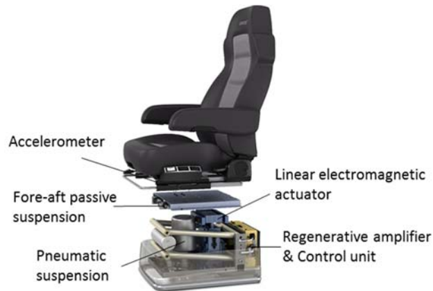
Figure 6. Anatomy of the electromagnetic active seat suspension system (BoseRide® System). The main components include the linear electromagnetic actuator used to suspend and control the vertical movement of the seat and fore/aft passive mechanical suspension.
