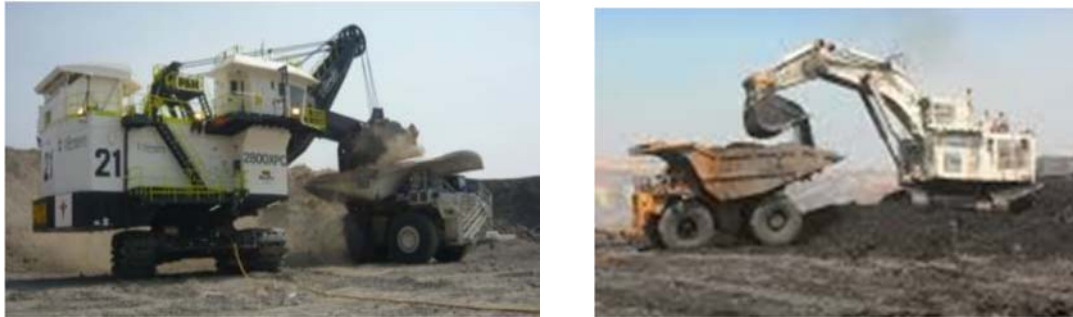
Figure 1. Typical heavy equipment vehicles (HEV), a shovel and load truck during a shock impulse loading scenario, not well captured with traditional whole body vibration exposure metrics
