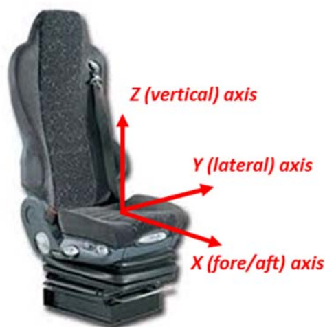
Figure 2. Coordinate system used to measure whole body vibration, as defined by ISO 2631-1:1997
