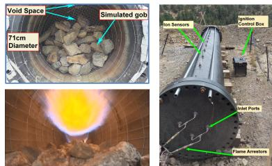
propagation velocities reducing run-up length to becoming fully turbulent with the enhanced potential of transitioning to detonation as the rock barrier length is increased.
