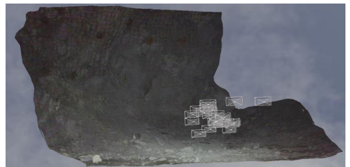
Fig. 13. 3D mesh of the S rib (top) and the N rib (bottom) of the 895-102 intersection at the Barrick Golden Sunlight Mine produced using Bentley ContextCapture from a video captured by a DJI M100. The gray boxes indicate the camera stations of the M100 while it was flying. On-board lighting was used.
