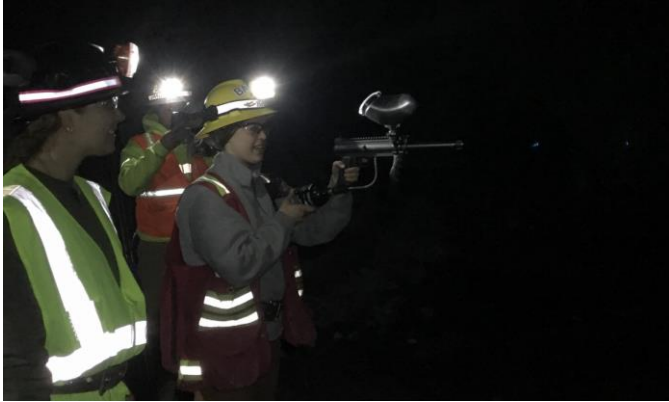
Fig. 10. Example of paintball marker in use for establishing control points. It was necessary to shoot multiple times at a single point because of dust on the ribs of the stopes and drifts.
