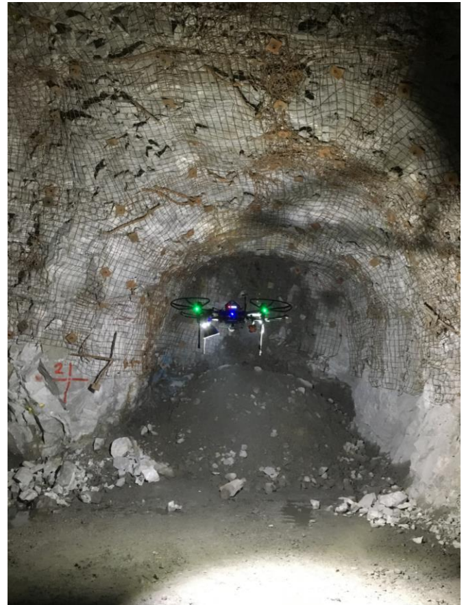
Fig. 3. The M100 hovering within the 895-102 intersection at the Barrick Golden Sunlight Mine. The UAV is approximately 2.75 m (9 ft.) off of the sill, and the blue light indicates that the downward-facing Guidance sensor is functioning properly and positioning the aircraft.
