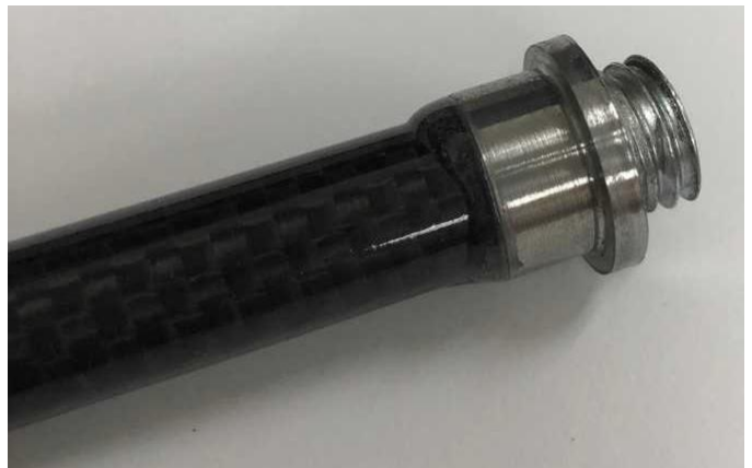
Fig. 3. Machined drain plug used to serve as UAV leg attachment piece.
