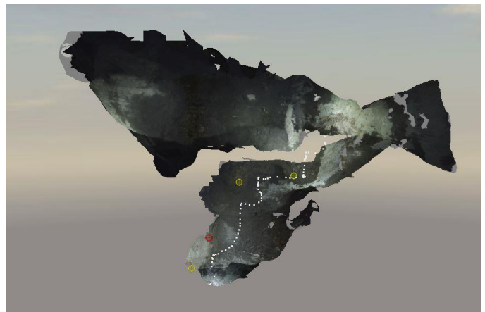
Fig. 11. ContextCapture model built from a UAV flight into the first drawpoint of the NEV stope at GSM (GCP1, 2, & 4 in yellow; GCP3 in red; white dots represent the UAV route).
