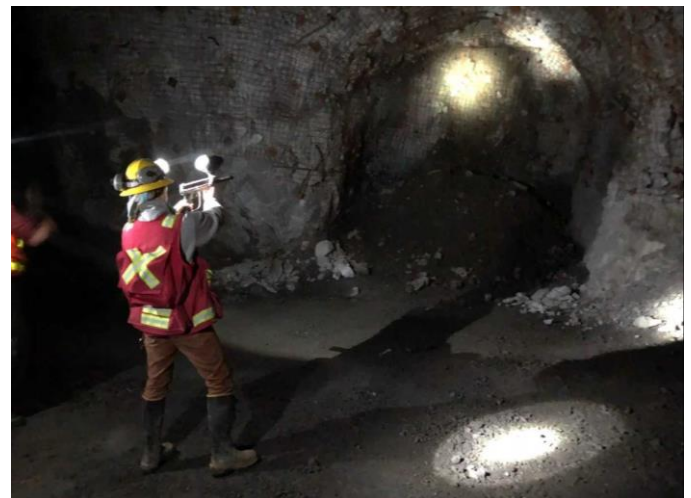
Fig. 5. Elizabeth Russell using the paintball gun to mark control points in areas that are out of reach.
