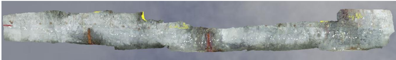
Fig. 10. Model of the 815-102 drift at GSM created using Bentley's ContextCapture.
