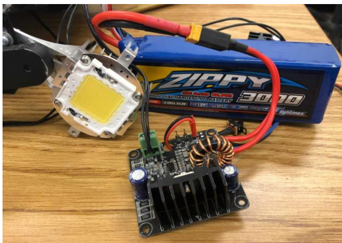
Fig. 2. Stratus Arm LED module used on the UAV.
