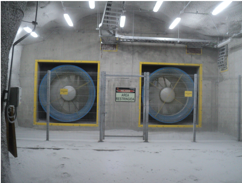
Figure 4.16: Underground booster fan installation (inlet side).
