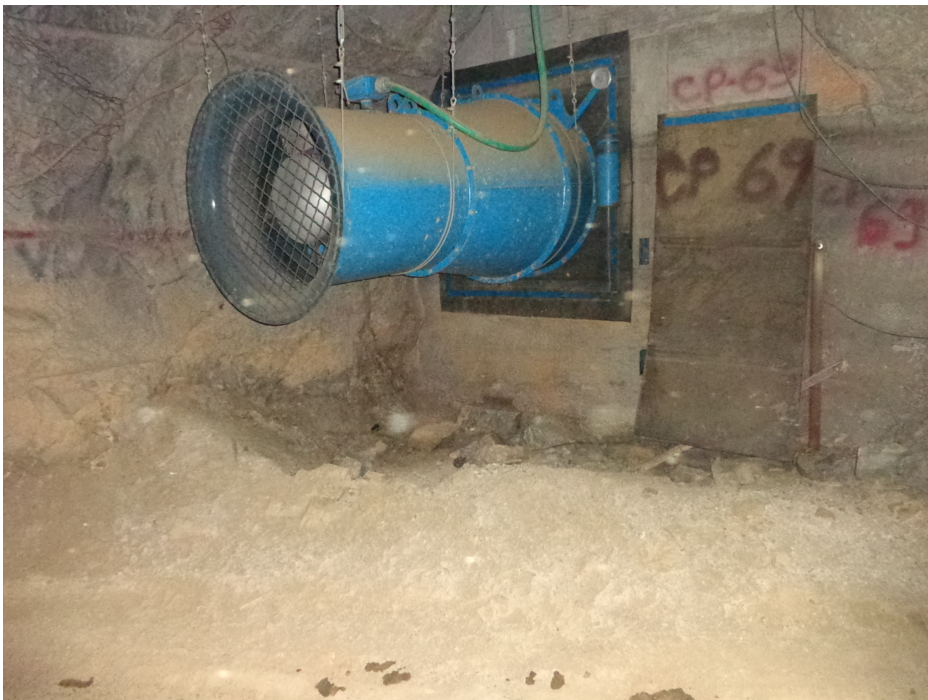
Figure 4.15: Underground booster fan for production panel with pressure-relief door.
