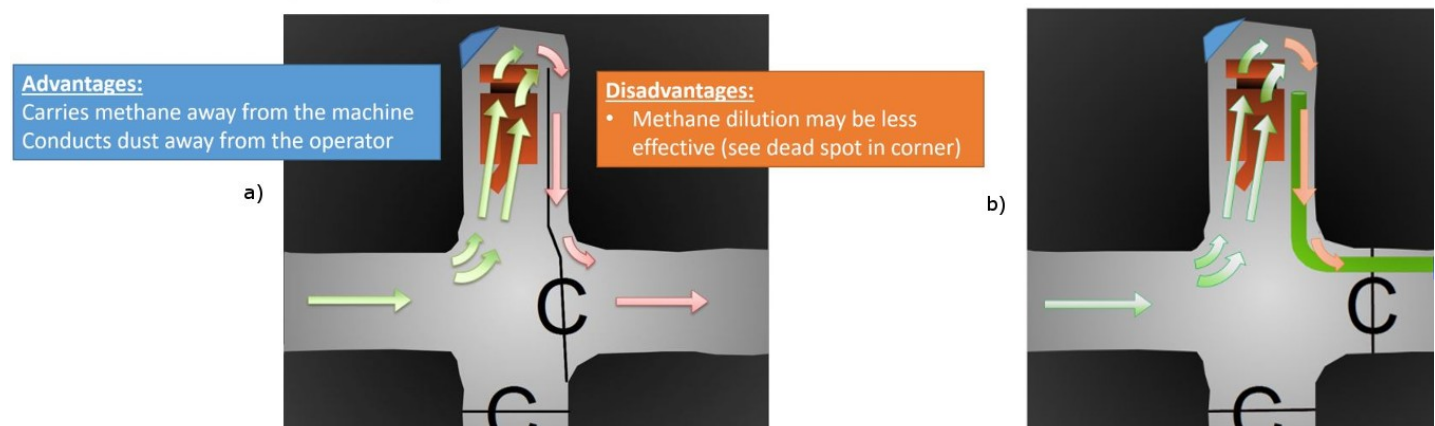
Figure 4.2 Exhausting face ventilation system (plan view).
