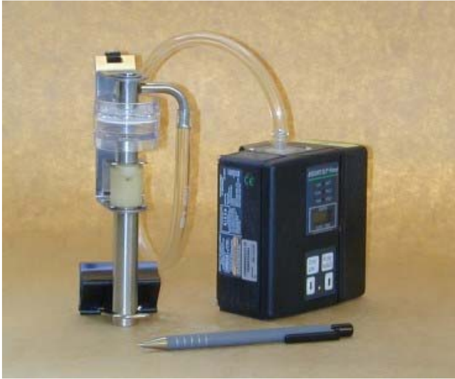
Figure 3.5: Typical Gravimetric Dust Sampling Train (NIOSH, 2010).
