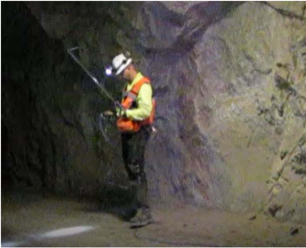
Figure 3.2: Pressure measurement being performed with a gauge and tube.
