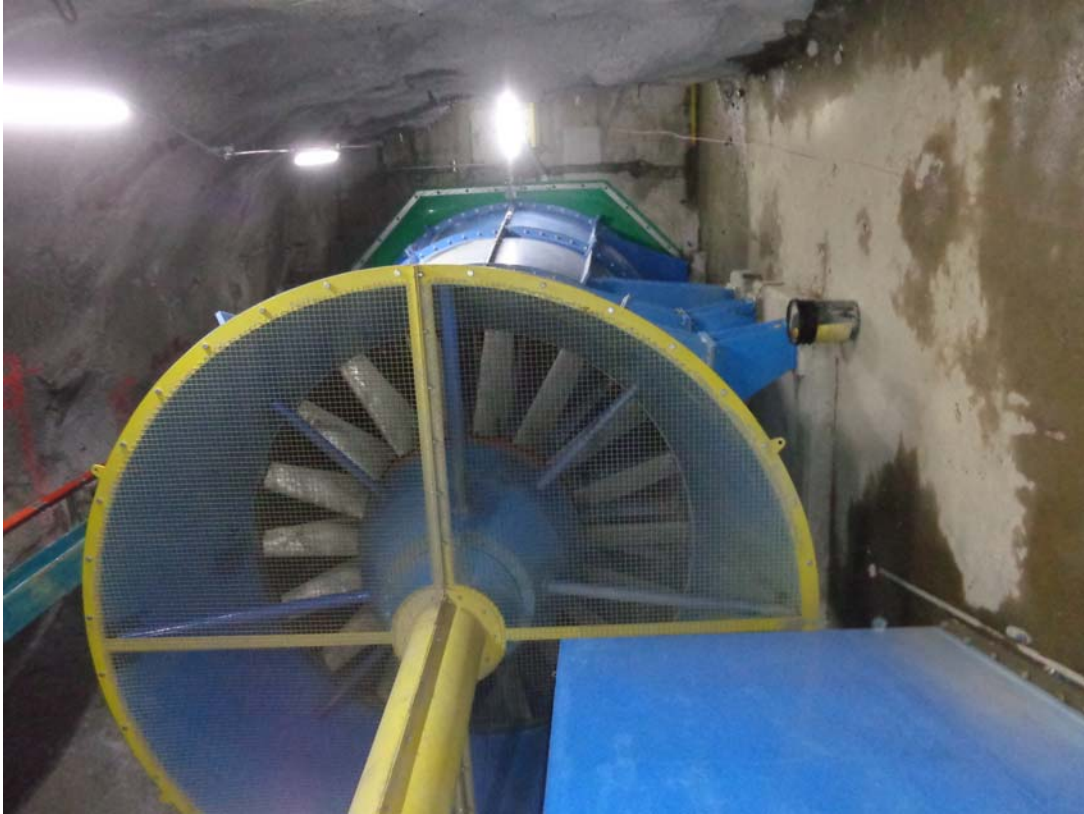
Figure 2.2. End of an axial flow fan being implemented as a mid-ventilation system booster
