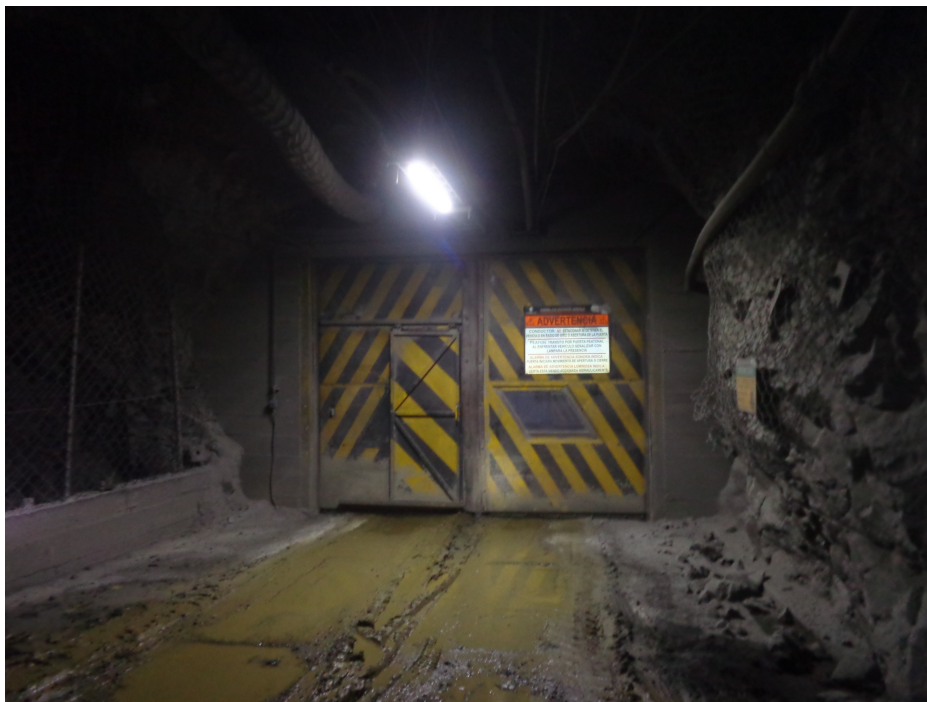
Figure 4.13: Underground Ventilation Control Door with mandoor and window.
