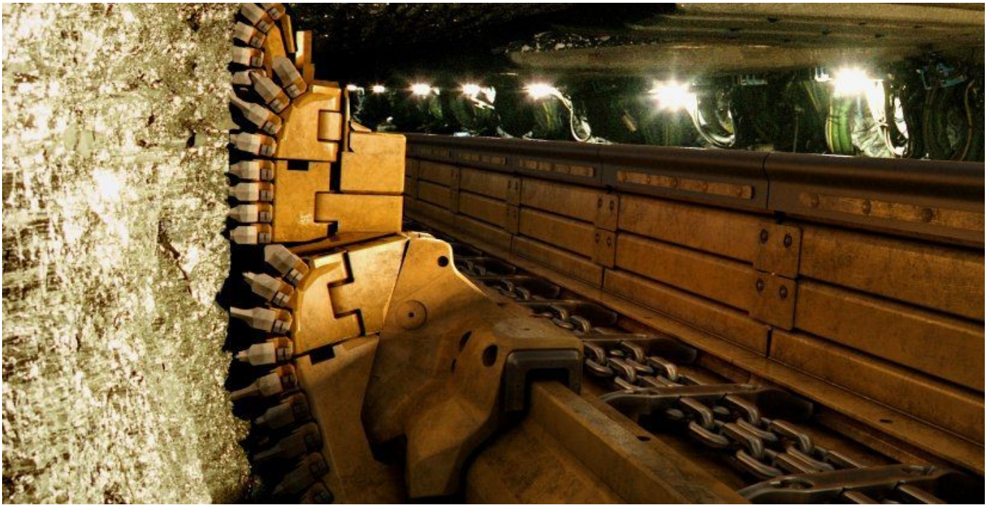
Figure 3.4. Plow longwall. The plow is shown to the left against the coal face, while the armoured face conveyor is shown towards the right. (Caterpillar, 2018 _( https://www.cat.com/en_US/campaigns/awareness/underground-plows-low-seam-coal.html ) )
