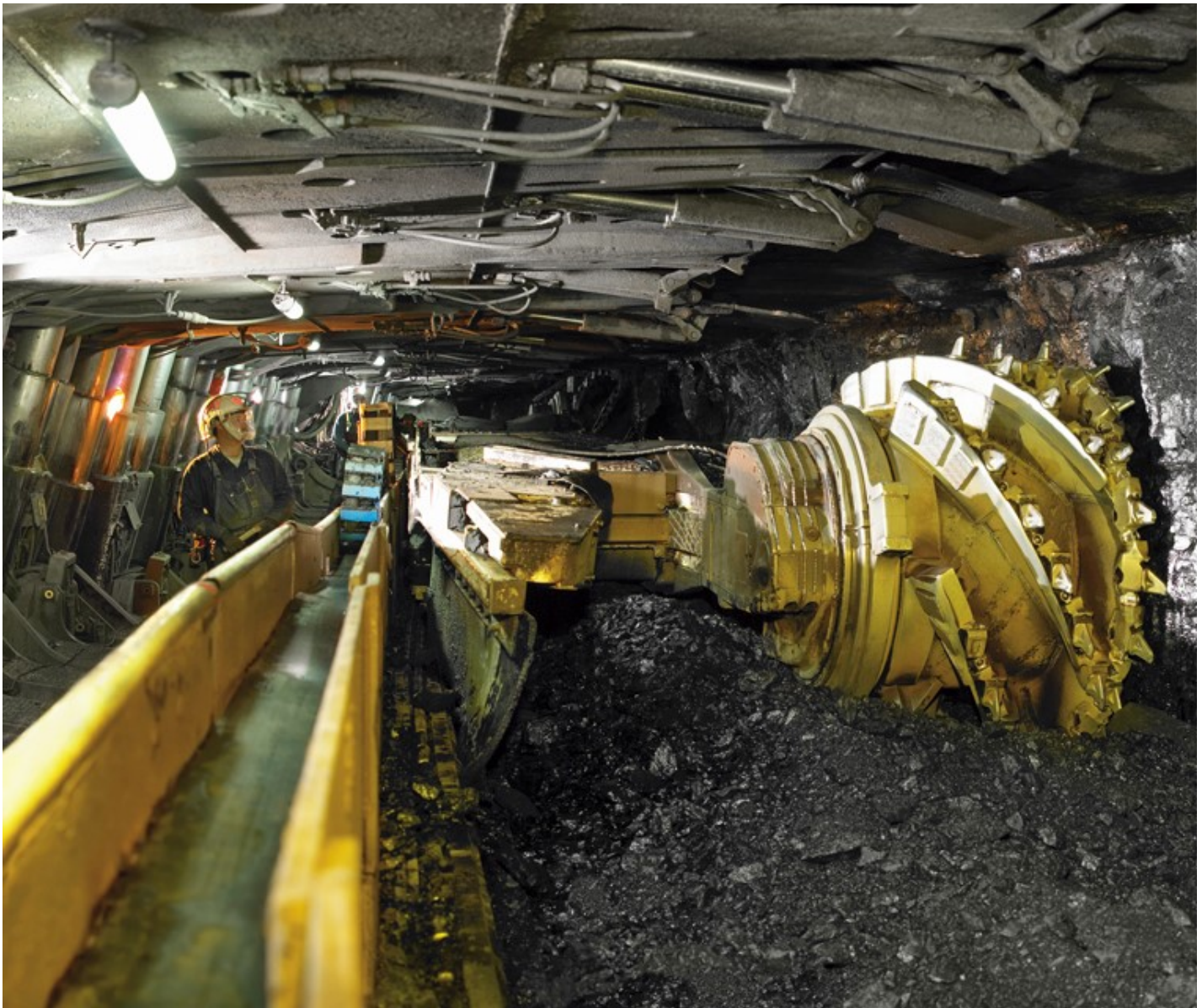
Figure 3.3. Longwall mining, shearing cutting drum to the left, notice the operator is wearing an air stream helmet "for protection against respirable dust. (NASA, 2015 https://landsat.gsfc.nasa.gov/assessing-longwall-mining-impacts-on-forests-above/ ).
