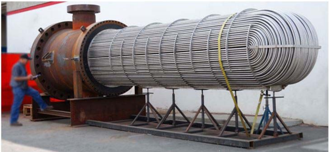
Figure 4.5: Shell and Tube heat exchanger (Actual).
