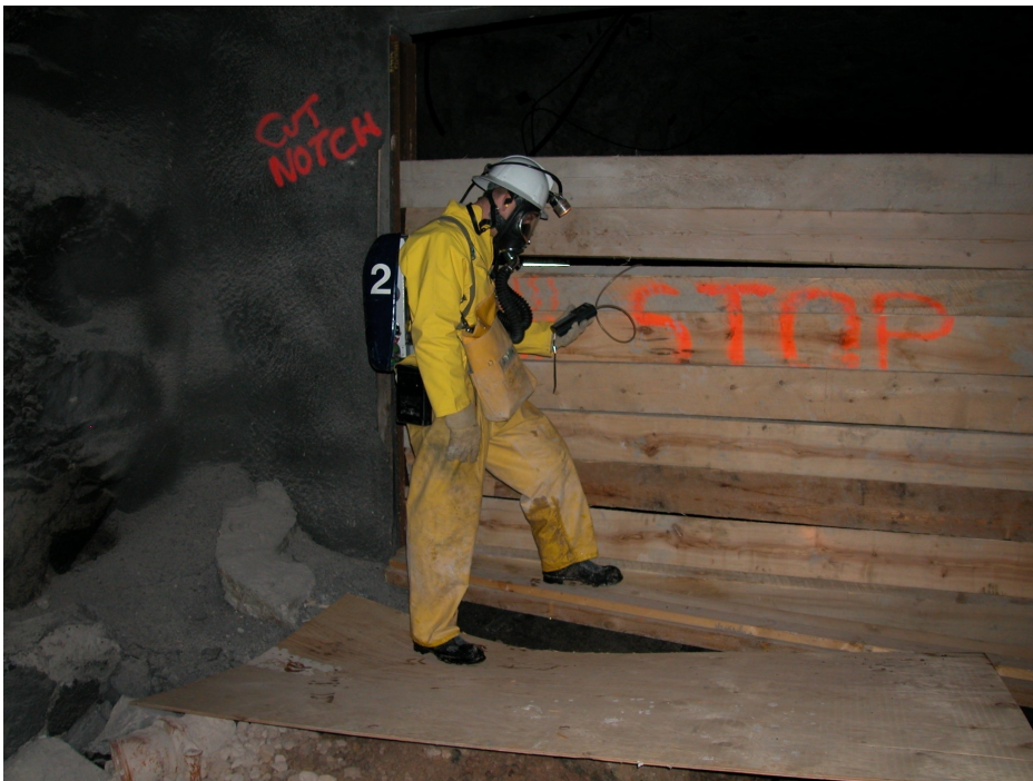
Figure 4.10: Drop-board regulator in an underground Uranium Mine.
