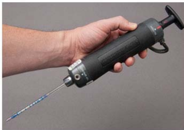
Figure 2.1. A stain detector tube attached to a hand pump ( OSHA, 2017b (https://www.osha-slc.gov/publications/1094345/pages/resources) ).
