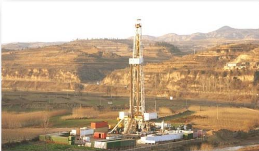
Figure 1. A drill rig for a vertical-to-horizontal multilateral well at an underground coal mine in China.
