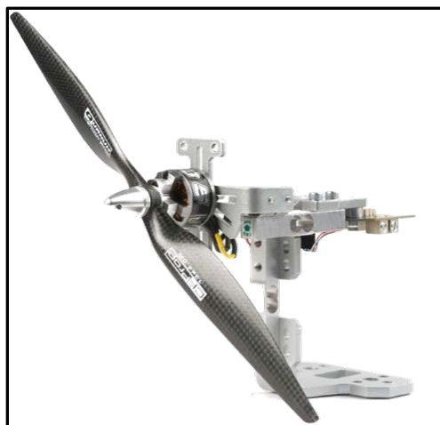
Figure 12: Apparatus to measure motor and propeller combination performance
