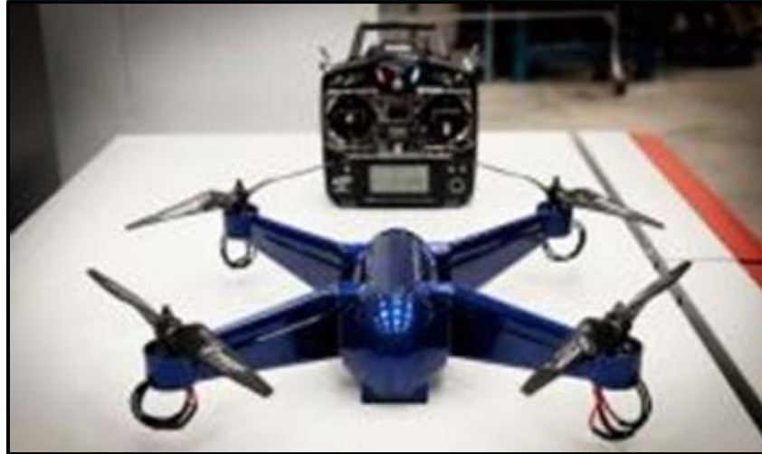
Figure 8: Nanyang Technological University 3D printed drone
