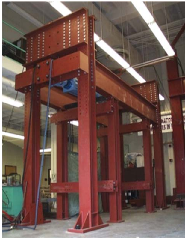
Fig. 34: MTS 810 materials testing setup.
