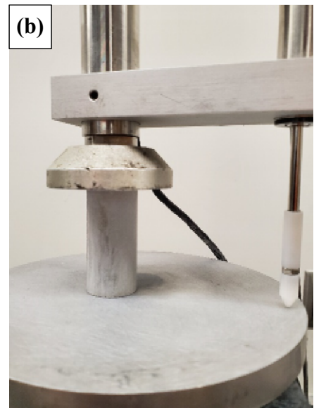
Fig. 8: (a) ELE Tri Flex 2 loading machine; and (b) Specimen under unconfined compressive loading.
