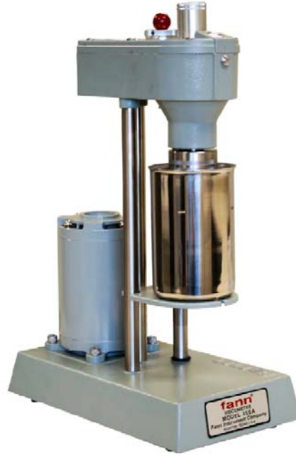
Fig. 6: Viscometer Fann model 35A.
