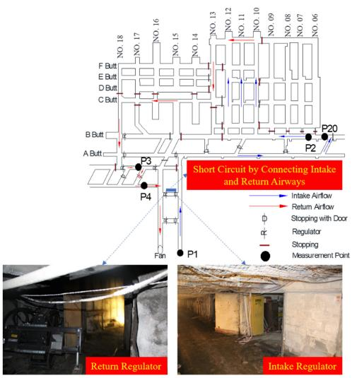
*Figure 4-21.* Location of the mine doors that were opened to create the short-circuit path.
