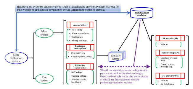
*Figure 4-7.* Illustration of the simulation approach used to investigate the ability of sensors in specific locations to detect developing problems.
