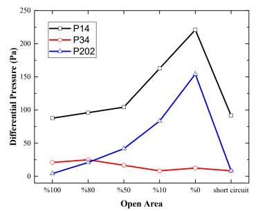
*Figure 4-28.* Differential pressure between monitoring positions with various interruptions.
