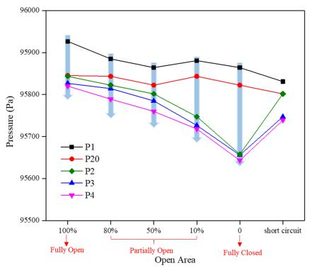
*Figure 4-24.* Pressure at monitoring positions with various ventilation interruptions.
