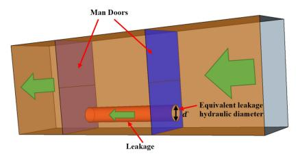
*Figure 4-14.* Illustration of airflow leakage through man doors in stoppings.
