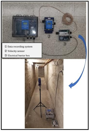
*Figure 10-4.* Airflow velocity system installed in the PSU-MVL.
