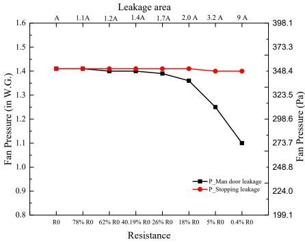
*Figure 4-16.* Results of fan performance at monitored spots in different resistance reduction cases.
