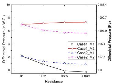
Figure 4-18. Differential pressure at regulators for each case and for different levels of resistance.
