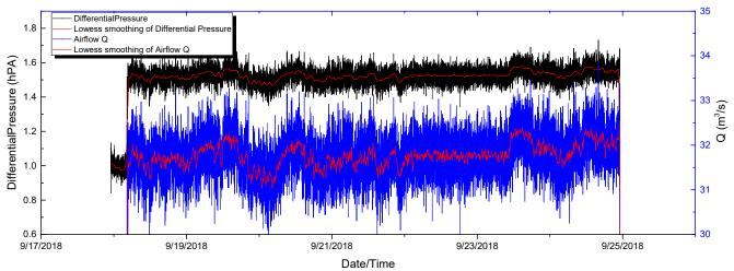
*Figure 4-4.* Comparison of velocity and pressure as surrogates of air quantity.
