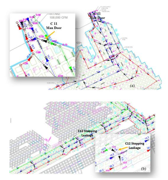
*Figure 4-13.* Man doors and stopping leakage positions on the mine map.
