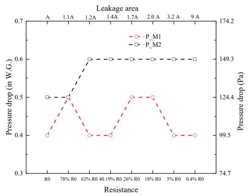
(b) Stopping air flow leakage at extended main (A - initial equivalent area and R<sub>0</sub> - initial resistance of leakage entry)
