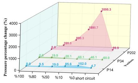
*Figure 4-29.* Pressure percentage change of differential pressure with reducing open area.
