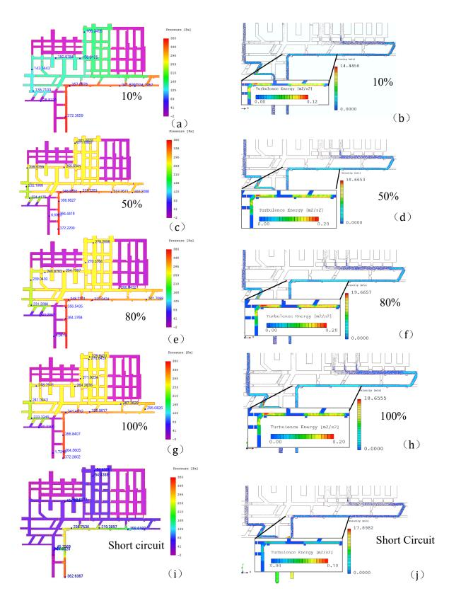
*Figure 4-30.* Pressure (Pa) and velocity profile with respect to various ventilation interruptions.
