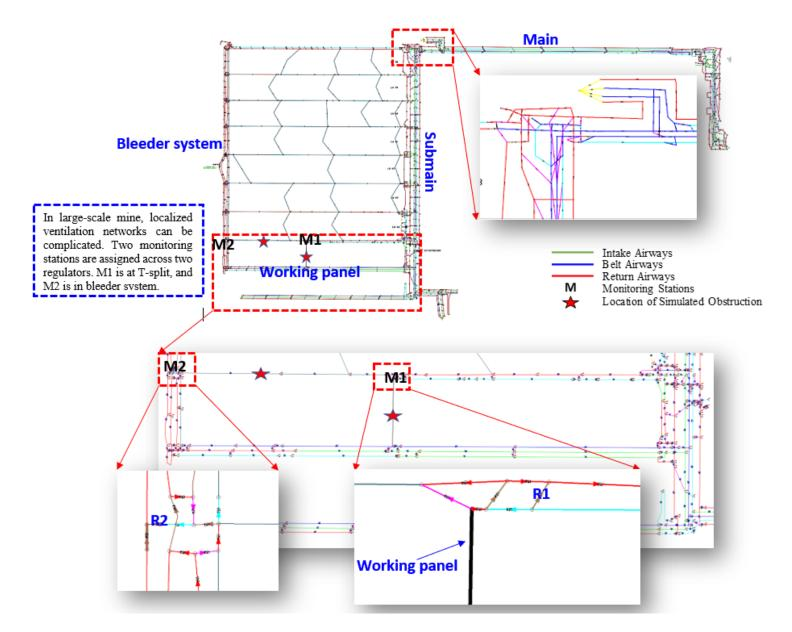
*Figure 4-177.* Large mine layout ventilation network with monitoring stations.
