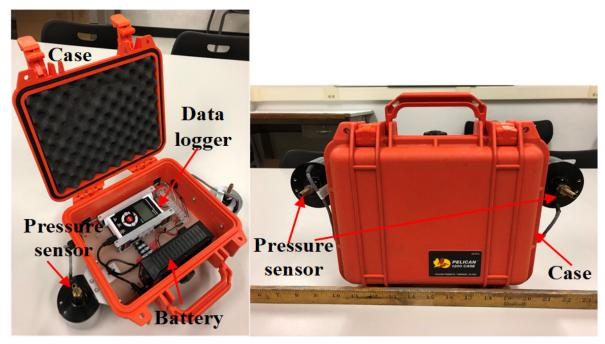
*Figure 4-2.* Differential pressure sensor with embedded data logger.
