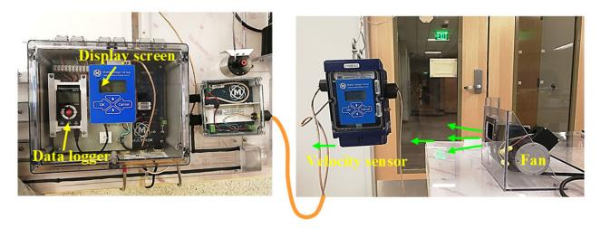
*Figure 4-1.* Velocity sensor with embedded data logger in the outstation. Note: The equipment is shown in the laboratory.
