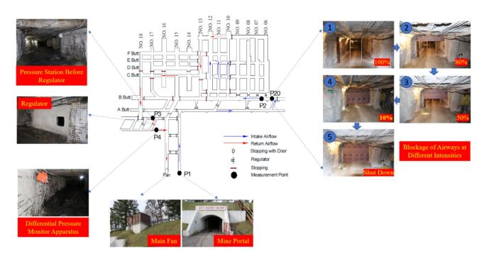
*Figure 10-3.* Safety research coal mine layout and ventilation monitoring stations.
