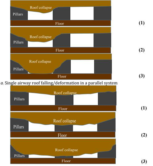
b. Coal pillar collapse-induced roof falling/deformation in a parallel airway system
