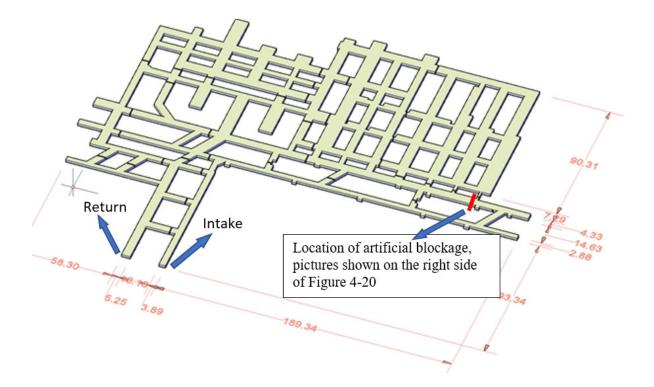
*Figure 4-23.* 3D CFD model of the Safety Research Coal Mine (unit-meter).
