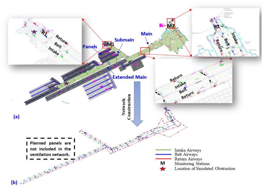
*Figure 4-10.* Small mine layout and corresponding ventilation network.
