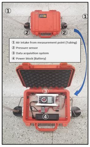
*Figure 10-1.* Pressure monitoring and recording system.
