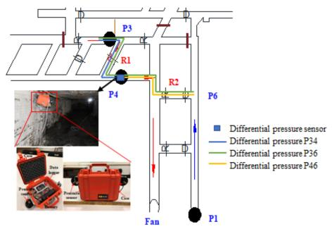
*Figure 4-22.* Differential pressure measurements between different monitoring stations.
