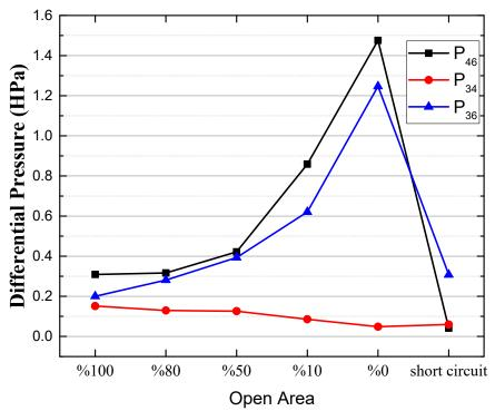
Figure 4-27. Differential pressure with various ventilation interruptions.
