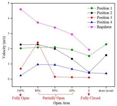
*Figure 4-25.* Velocity at monitoring positions with various ventilation interruptions.
