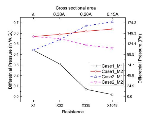
*Figure 4-11.* Plot of differential pressure at two monitoring regulators in roof fall incidents.
