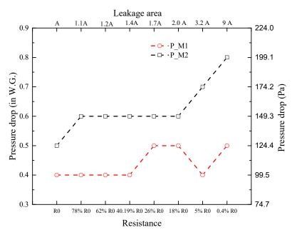
(a) Case study results of main door air flow leakage (A - initial equivalent area and R<sub>0</sub> - initial resistance of leakage entry)
