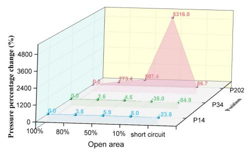
*Figure 4-31.* Pressure percentage change with respect to various ventilation interruptions.
