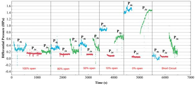
Figure 4-26. Differential pressure data across regulators with various ventilation interruptions.
