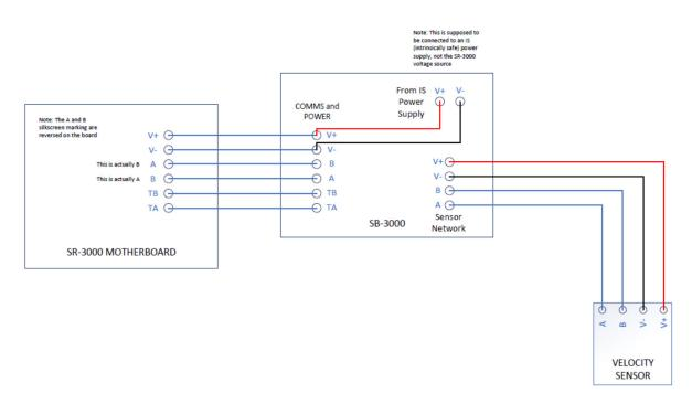
*Figure 10-5*. Velocity monitoring and recording system wiring schematic.
