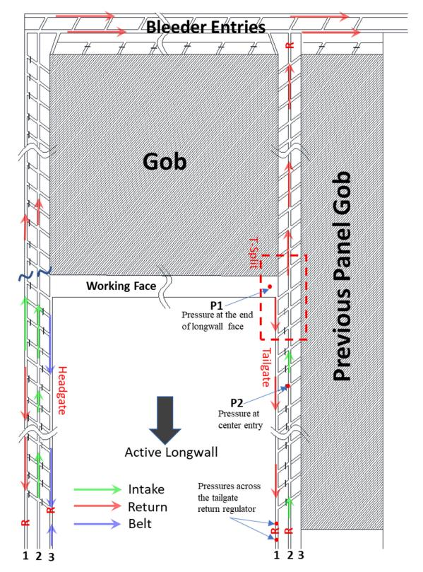
*Figure 4-6.* Placement of the pressure transducer and monitoring points to serve as a sentinel for the t-split.
