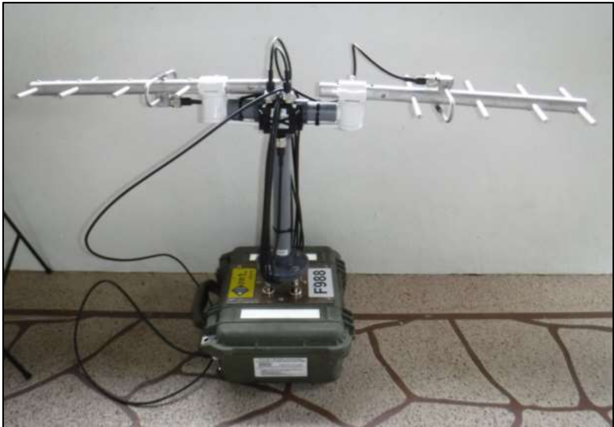
Figure 13: A directional IWT Portable Mesh Node (PMN) as deployed is about 2 feet high and 4 feet across.
