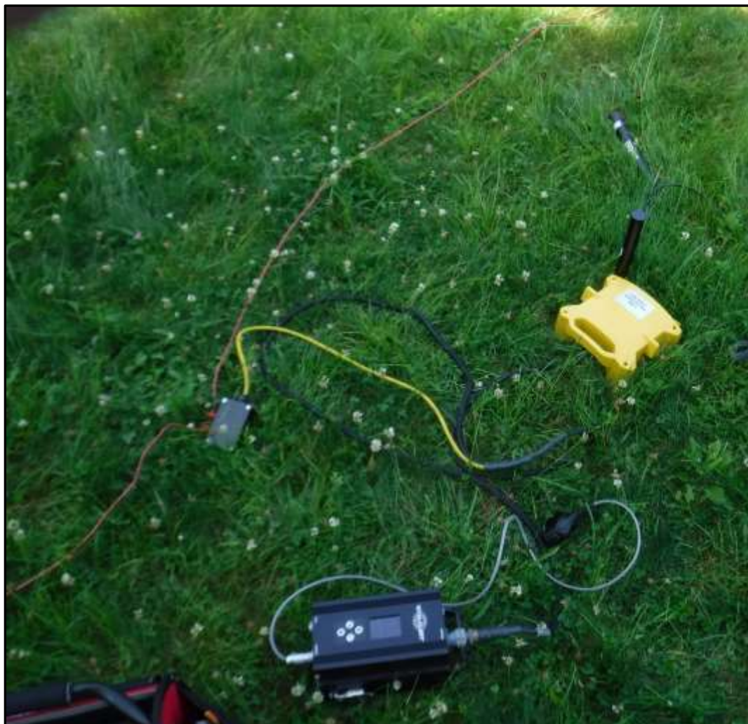
Figure 41: Remote VA equipment on June 26, 2019. The yellow unit is the VA receiving antenna connected to the black VA transceiver at the bottom of the photo. The VA 100-foot transmitter antenna is the red wire running diagonally across the left side of the photo.
