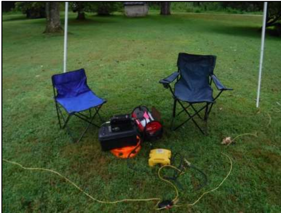
Figure 65: Close-up photo of the remote unit VA equipment at UG1 on August 7, 2019. The yellow wire is the remote unit's 500-foot circumference transmitter antenna.
