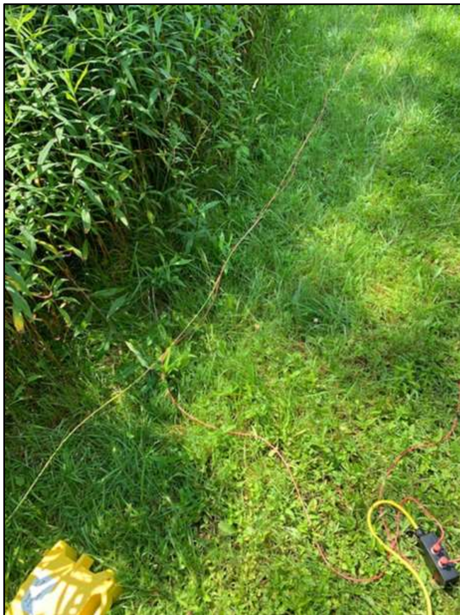
Figure 42: Photo showing the red 100-foot VA transmitter wire placed adjacent to the yellow 16-gauge linear conductor wire.
