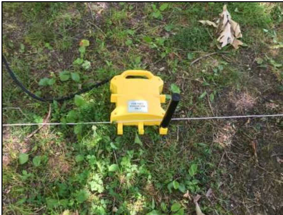
Figure 50: Close-up photo of the optimum placement of the VA receiving antenna and conductor wire for inductive communication.
