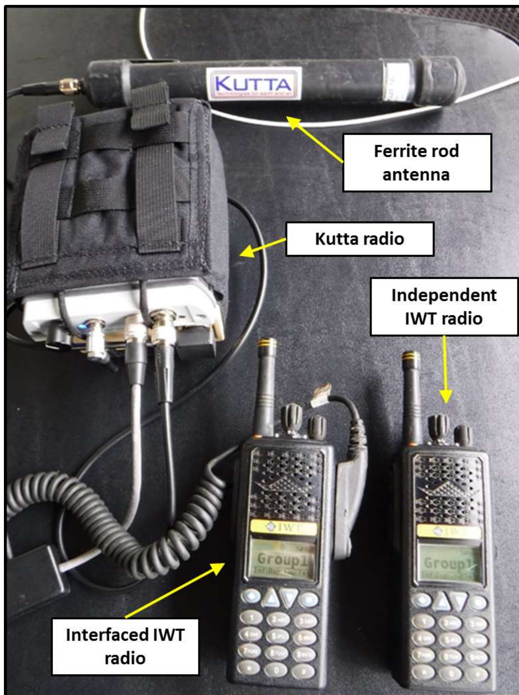
Figure 34: The base station equipment for the initial IWT/Kutta system interface test using a ferrite rod antenna.
