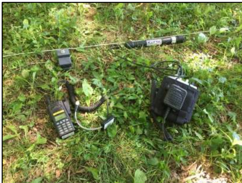
Figure 43: Kutta base station equipment with ferrite antenna placed parallel to the 12-gauge wire. The IWT radio interface and inductive clamp are not attached to the Kutta transceiver.
