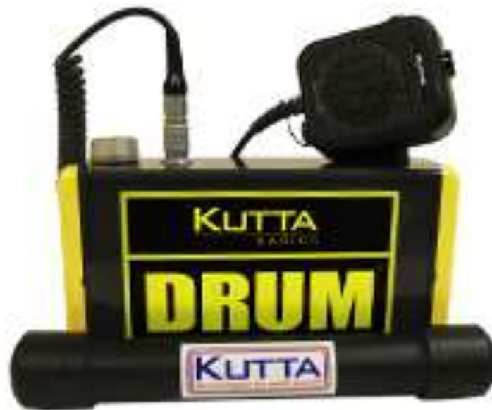
Figure 3. Kutta DRUM transceiver unit with its cylindrical antenna in the foreground
