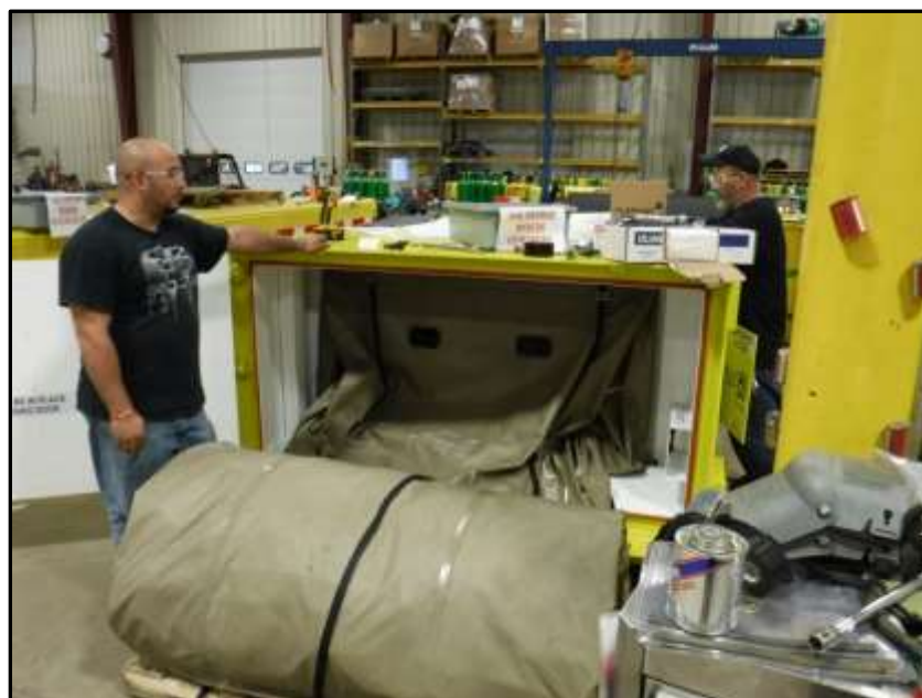
Figure 26: Insertion of a tested fabric tent assembly being in a new protective storage and transport unit.
