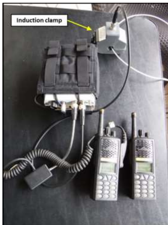
Figure 36: The Kutta MF induction clamp substituted for the rod antenna and placed around the wire.
