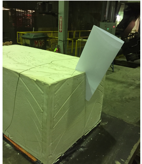
Figure 2. Sheet of paper place in macro fracture of seal material.
