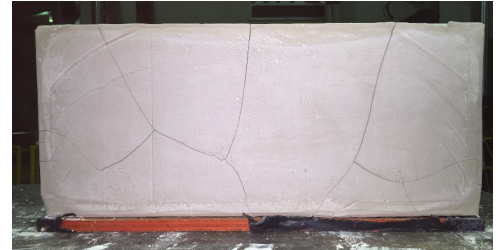
Figure 1. 28 in by 12 in block of seal material showing macro-scale fractures.
