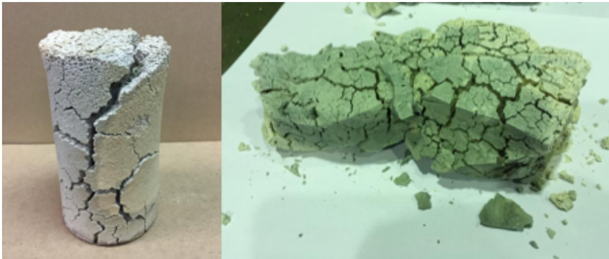
Figure 1. Pumpable material exposed to air for 24 hours. (On right specimen size is 7 x 12 inches and 2 in lab core on left).
