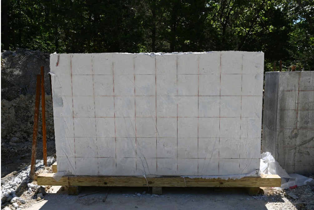
Figure 3.18. Unreinforced Pumpable Cementitious Seal
