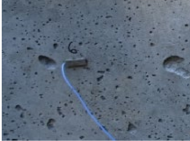
Figure 3.21. Strain Gauge on Rear Face of a Seal
