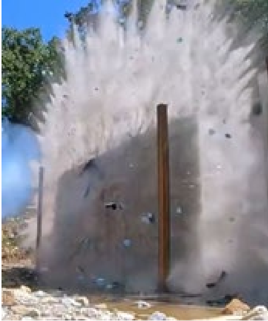
Figure 4.13. 30-lb. Concrete impact comparison between seal material types. Left is harder seal material where concrete projectile is pulverized resulting in no penetration. Right is softer seal material with significant penetration with concrete slug still inside seal.
