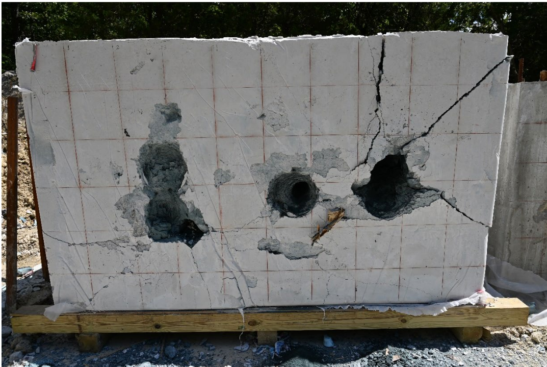
Figure 4.10. Unreinforced Cementitious Seal, Post-Test
