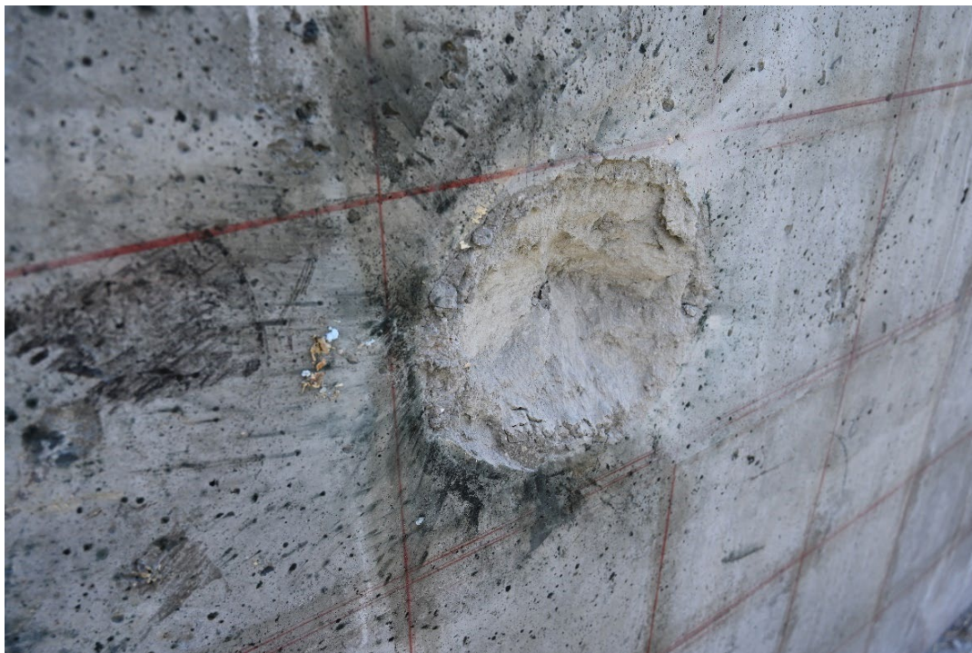
Figure 4.7. 30 lb. Steel Slug Impact Site
