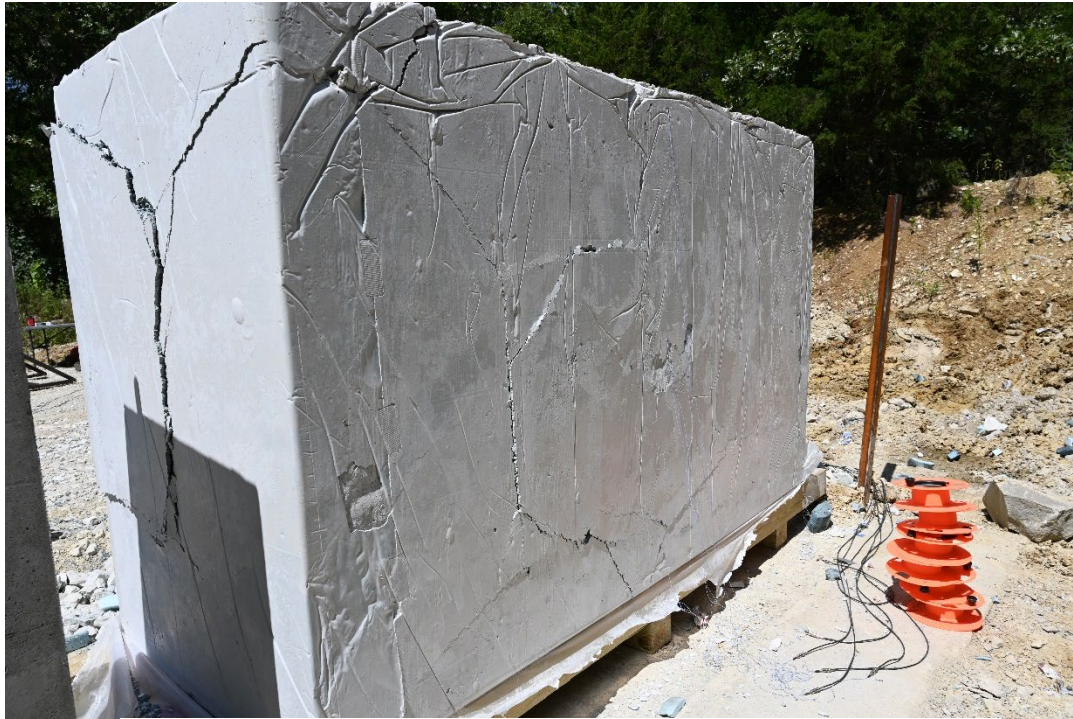
Figure 4.12. Unreinforced Pumpable Cementitious Seal, Rear
