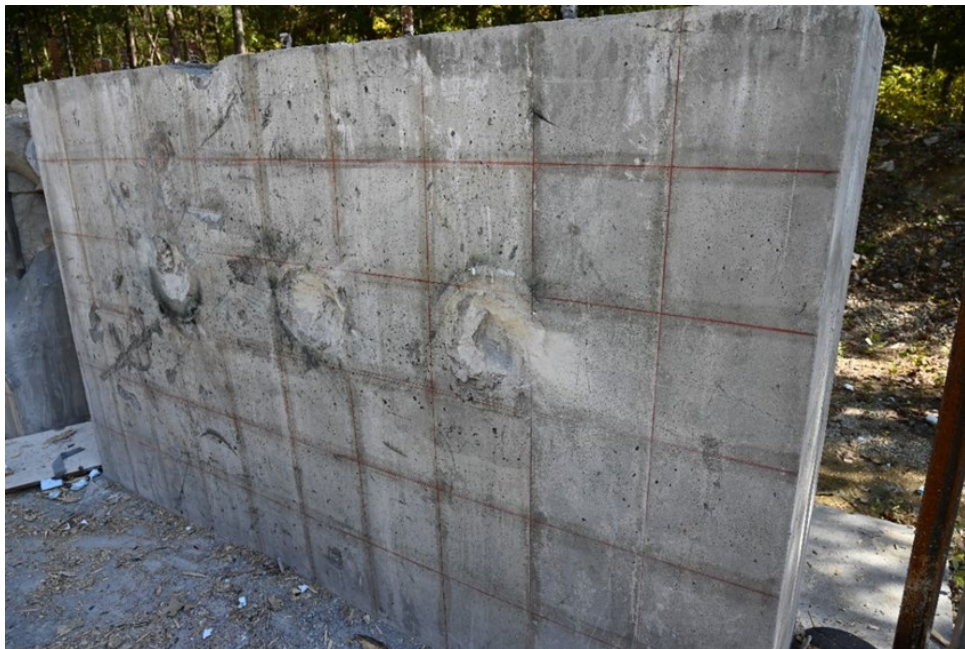
Figure 4.6. Reinforced Concrete Seal, Post-Test
