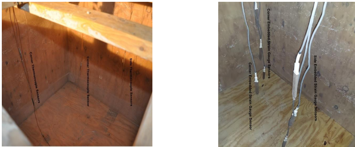
Figure 3.10 Strain gauges and thermocouple sensors before pouring the mine seal mixture
