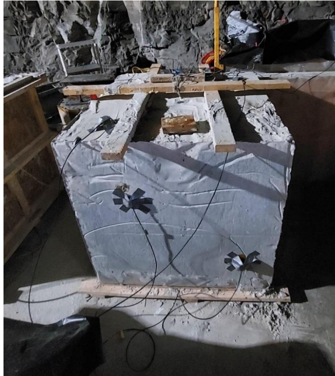
Figure 4.49 Sensors installed on the sample of Mixture D (Company 1 – Out of Spec)
