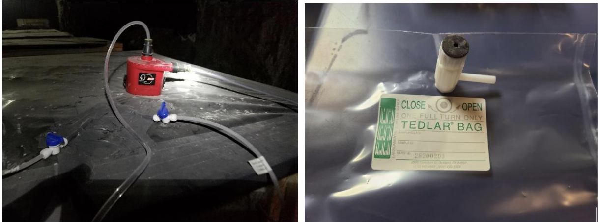
Figure 3.6 Vacuum pump system, sampling ports, and TEDLAR® gas sample bag
