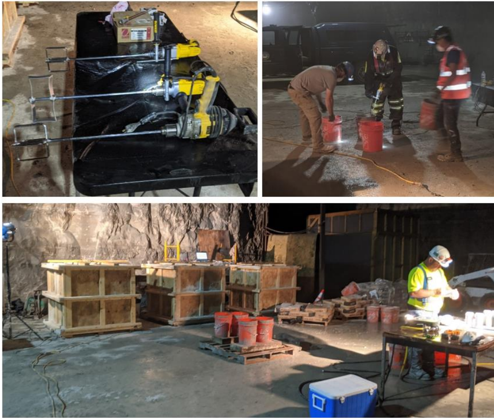
Figure 3.21 Manual mixing and pouring for additional sample (Company 1 – Mixture A (Within Spec) & Mixture D (Out of Spec) – manual pouring)
