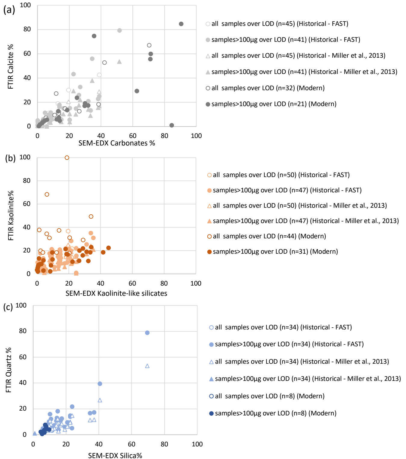
Figure 3. FTIR-derived mass % of (a) calcite, (b) kaolinite or (c) quartz versus SEM-EDX derived mass % of (a) carbonates, (b) kaolinite-like silicates, or (c) silica. Results for modern and historical dust samples are shown separately. The open points show all samples; the solid points show samples with total mass > 100 µg.
