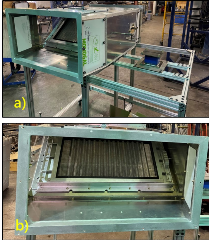
Figure 132. a) Custom-built mesh housing section b) The vibrating mesh configuration supplied by the Virginia Tech team.
