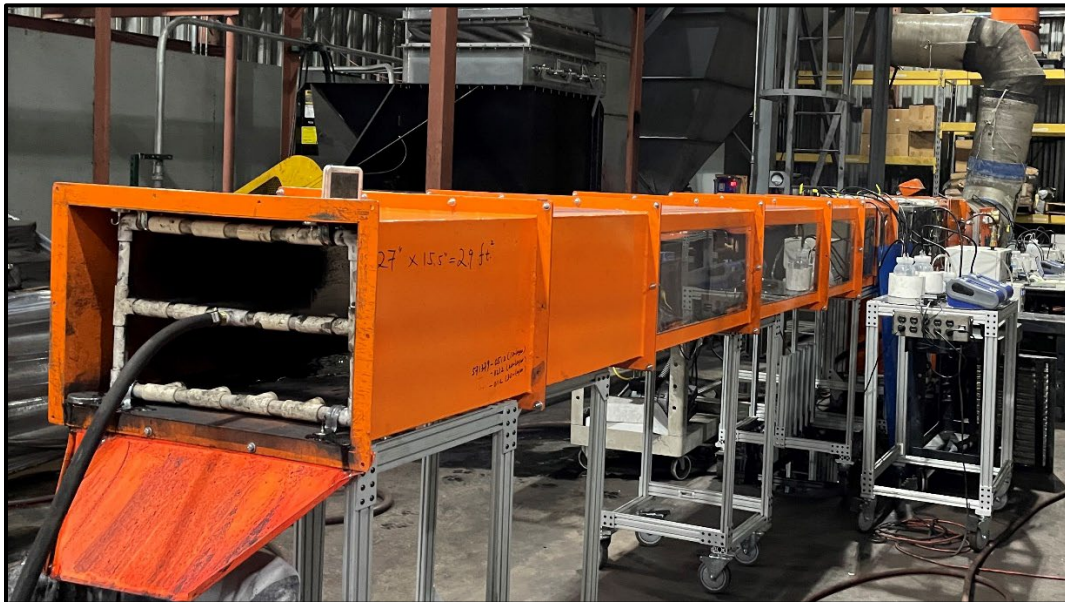
Figure 131. Standalone dust scrubber unit at the NIOSH Dust Gallery.
