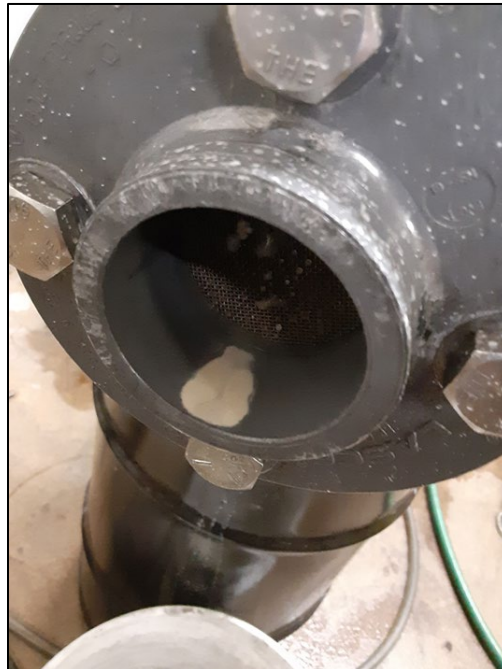
Figure 78. A photo of a filter assembly after a spray of granite slurry on a filter pack with 8 layers of hydrophobic 100-mesh wire meshes.
