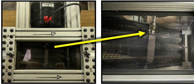
Figure 98. Clamping mechanism between the shaker's actuator rod and mesh screen.
