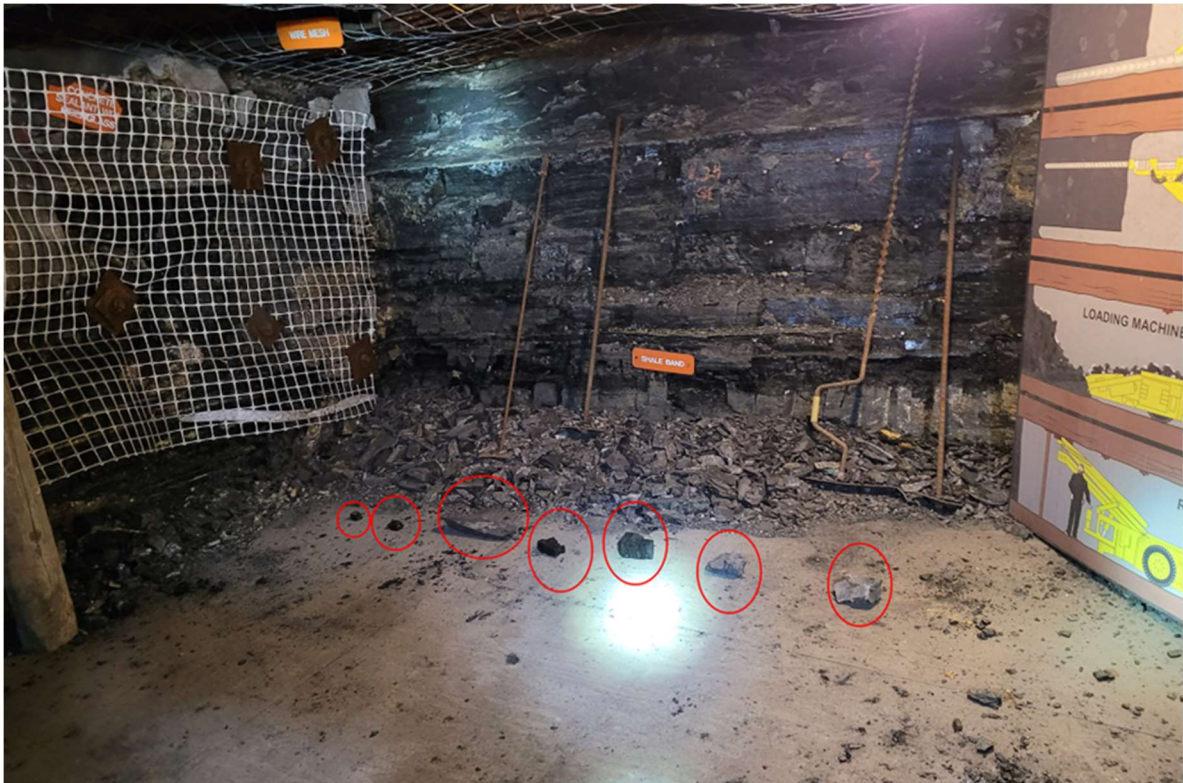
Figure 3.2. Artificially induced rock falls, seven rock pieces, on the entry floor.
