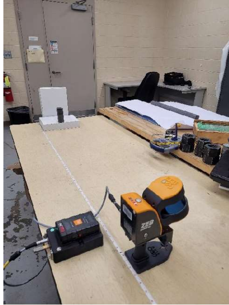
Figure 3.6. Laboratory experiment set up for classification of lithologies according to the intensity values.
