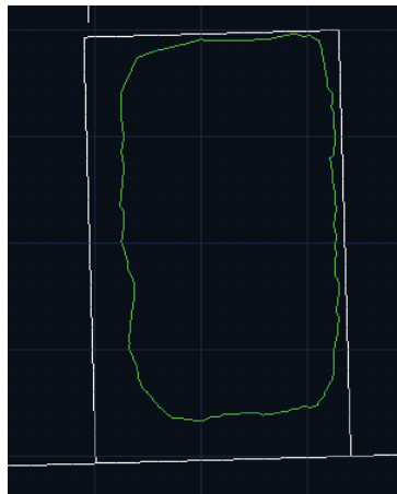
Figure 12: Selected pillar map design and LiDAR scan comparison
