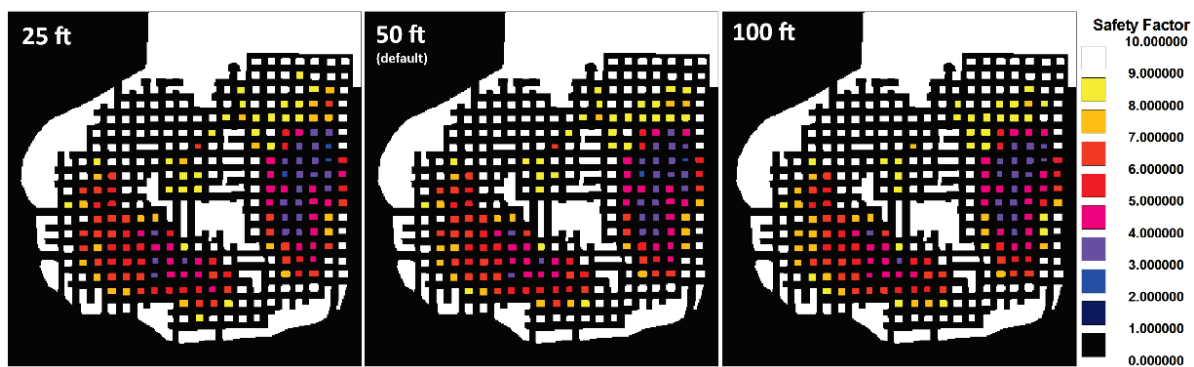
Figure 24: Safety factors obtained with different lamination thicknesses
