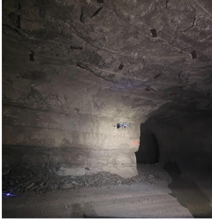
Figure 21 Mapping test on the Ohio mine wall
