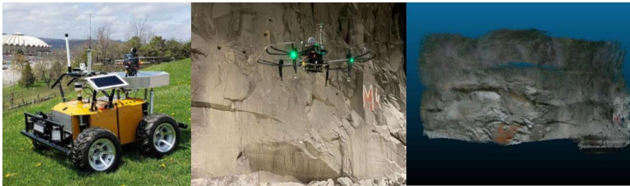
Figure 7 Robotic system developed for mining inspection. Left: the UGV with the UAV in the landing platform; Center: UAV autonomous surveying a pillar; Right: 3D photogrammetry model obtained from the survey.
