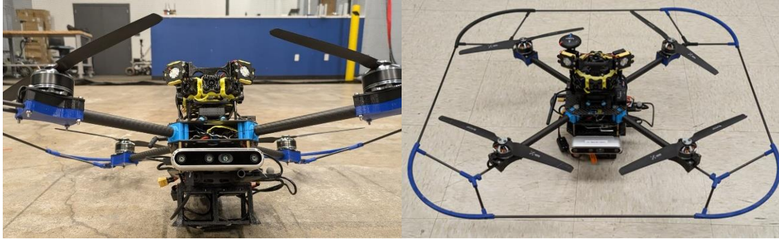
Figure 13 Mine Drone V2, with an extended frame and oversized propellers, equipped with a full Teratower array and independent front and downward-facing light sources, and carrying a RealSense D455 as payload.
