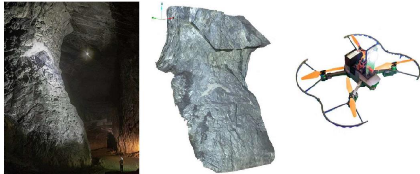
Figure 4 Drone-based pillar survey for photogrammetric modeling (after, Bishop, 2022)
