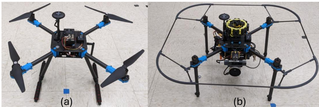
Figure 12 (a) Basic drone platform used in the project; (b) Mine Drone V1, equipped with a T265, L515 and Teratower laser sensor.
