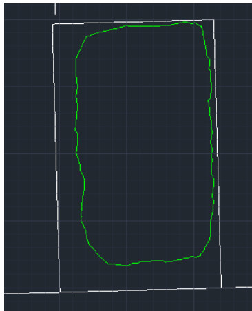
Figure 65 Selected pillar map design and LIDAR scan comparison
